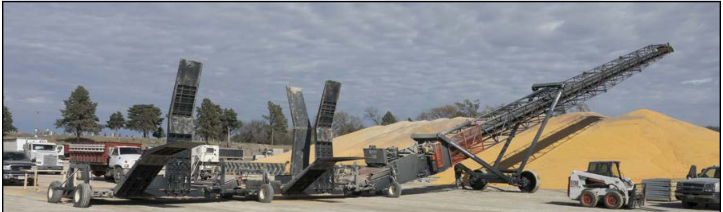
Drive-over unloading conveyors are available in single or double (shown) drive-over configurations
