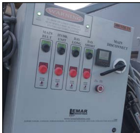
LeMar® Transport Conveyor Control Panel
