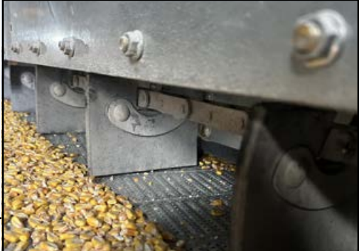
Paddle Design moves grain with less shear and impact.
