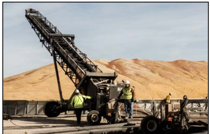
Brock's LeMar® Transport Conveyor can pile grain to 38 feet (11.5 m) peak height and reach the middle of a 150-foot (45.7-m) wide bunker.
