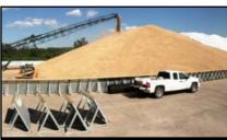
Aeration Wall provides full round, 360-degree, air entry for balanced aeration of the grain mass.
