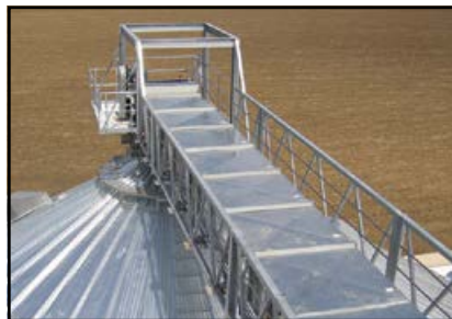
Handrail Truss comes in standard widths of 30-108 inches (762-2743 mm) and maximum span of 125 feet (38.1 m).
