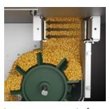
isolates grain moisture measurements for ultimate accuracy.
