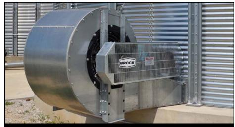
Factory-balanced Centrifugal Wheels provide smooth, efficient fan operation aided by Brock's cable suspension mounts for hanging fans from the bin's sidewall. Cable suspension makes it easier to clean under the fan and is 50% less than the cost of a concrete foundation. Concrete foundation option is available.
