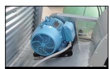
Fan Motor mounts on transition housing to eliminate the typical added suspension needed for the motor along with potential strain on fan motor bearings. Future fan motor upgrades to higher horsepower are also easier.
