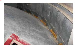
Brock's unique self-cleaning plenum floor design allows fines, dirt and bees' wings to recycle back into the grain safely while also reducing routine cleaning maintenance.
