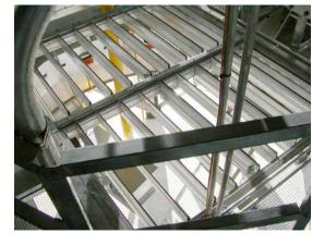
Fresh air along with electrical conduits and gas piping enter at the bottom of the dryer and not through the grain columns. This promotes even grain flow and efficient drying. Air inlet louvers are adjustable to control the volume of cool air entering the dryer.
