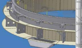
**GENTLE GRAIN UNLOADING SYSTEM** Brock's innovative and gentle Circular Drag Grain Unloading System (patented) evenly meters grain from the grain columns and gently delivers it to the unloading point at the perimeter of the dryer. The speed of the unloading system is automatically adjusted to allow for moisture variations in the incoming wet grain.
