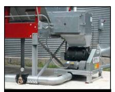
**SUPER-AIR® Pneumatic System** uses positive pressure to help move grain to multiple bins with just one power source. Choice of 4-, 5- or 6-inch (102-, 127- or 152-mm) diameter systems and capacities ranging up to 2,250 bushels (57.2 metric tons) per hour.
