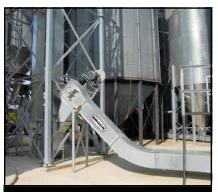
**Drag Conveyors** are available in a range of styles and sizes to suit any operation's needs. Capacities range up to 42,800 bushels (1,087 metric tons) per hour.
