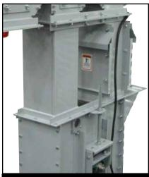
**Trunking Flanges** are solid welded inside and out for durability and performance. Components are fixture-welded to ensure better accuracy and easy construction in the field. Trunking is always galvanized as the standard finish.
