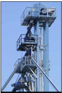
Elevator Head Platform wraps around the front of the head. This offers ample access for inspection and service. Galvanized steel, urethane or high-energy urethane liners for the head section are available based on your specific application.
