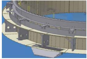
Brock's innovative and gentle Circular Drag Unloading System (patented) evenly meters and delivers the grain to a discharge point at the perimeter of the dryer.
