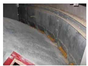
Brock's unique self-cleaning plenum floor design allows fines, dirt and bees' wings to recycle back into the grain safely while also reducing routine cleaning maintenance.
