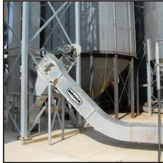
Brock GrainDrive™ Curved Incline Drag Conveyors
