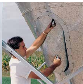
Optional ACCESS PLUS® Hopper Access Door (patented)
