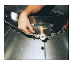
A manual holddown clip is provided for added security when working around or inside the bin or fill hole area.
