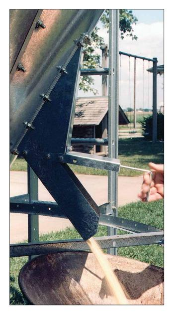
Brock's unique Hopper Valve Kit gives an alternate way to easily get small amounts of feed or other stored materials out of a hopper-bottom bin or silo. This easy access is important when a small quantity of the stored material is needed at a location not serviced by the auger system.
